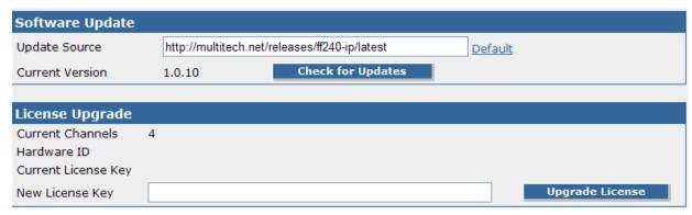
There may be occasions where features are refined or added to the FF240-IP unit. Such features will be available through updating of the software that exists in the FF240-IP.
